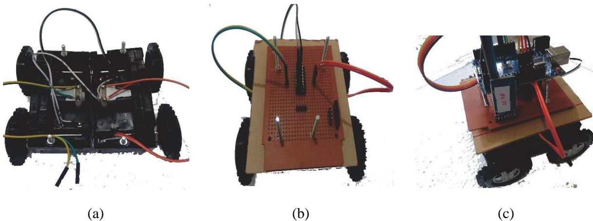
**Figure 2.** hardware of mobile robot based on smartphone (a) actuator, (b) motor driver and (c) mobile robot
