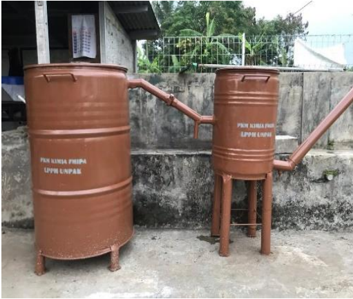
Figure 5. Micro installation for making liquid smoke
