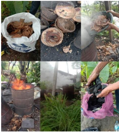
Figure 1. Conventional coconut shell charcoal making process
